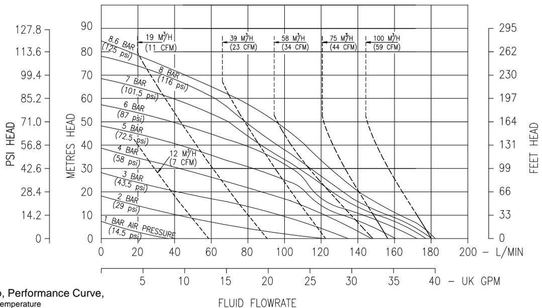
B2505 Metallic Pump, Performance Curve, based on water at ambient temperature
