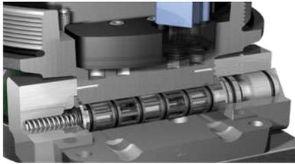
The Axiom's pneumatic valve system consists of a low-power pilot that drives the main high-flow spool valve. Pilots may be selected for conventional or bus networking applications. Both stages of the pneumatic valve system have been designed for long life, high tolerance to air line contaminants, and ease of maintenance should components become fouled.
