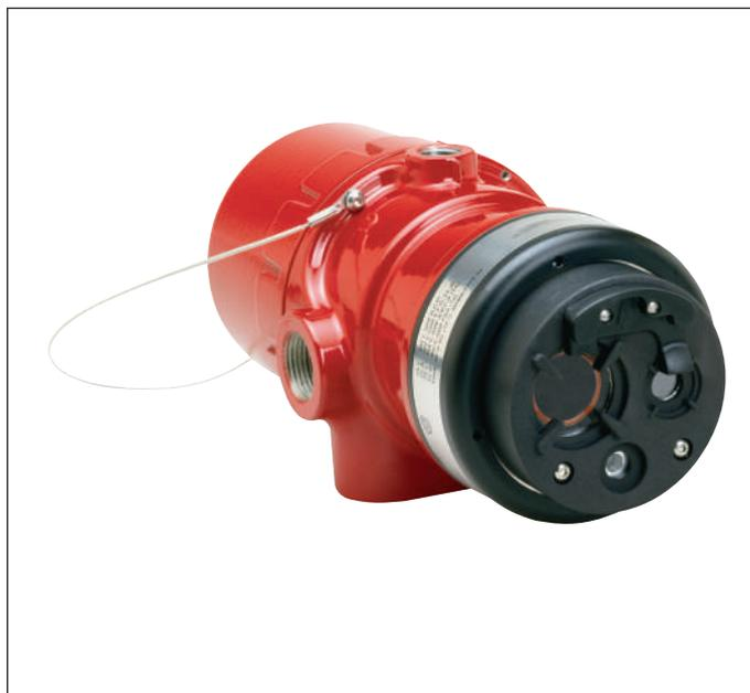
The standard output configuration includes fire, fault and auxiliary relays. An optional 0 to 20 mA output with HART can be provided in addition to the three relays. Auxiliary relay and 4 to 20 mA output are not available with the pulse model. A tricolor LED on the detector faceplate indicates normal condition and notifies personnel of fire alarm or fault conditions.
