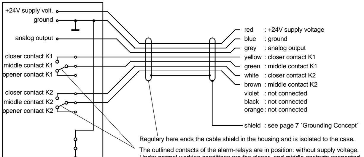
Regularly here ends the cable shield in the housing and is isolated to the case.
