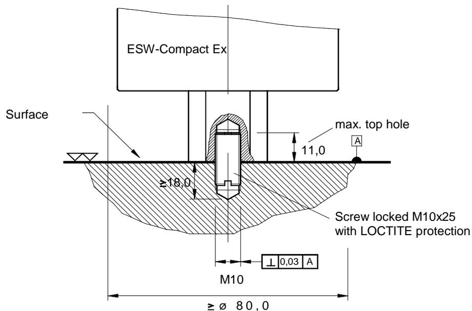
The ESW<sup>®</sup>-Compact/Ex will be mounted via one threaded pin AM10\*25 per DIN 913 on the machine to be monitored.
