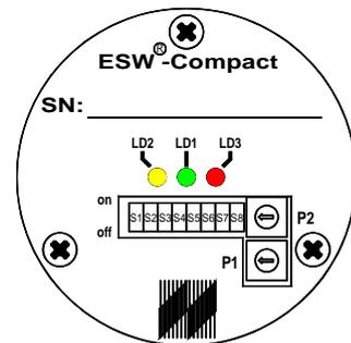
Upon execution of the self-test function, it’s absolutely necessary to return the switch S8 to the position OFF in order to ensure the proper function of the ESW<sup>®</sup>-Compact/Ex. The yellow LED must darken and current has to return to his normal value. In case the yellow LED is lighting and a higher output current is flowing, without of activation of S8, than the electronic recognize one sensor defect and starts alarm, because the electronic is continuously monitoring the sensor.
