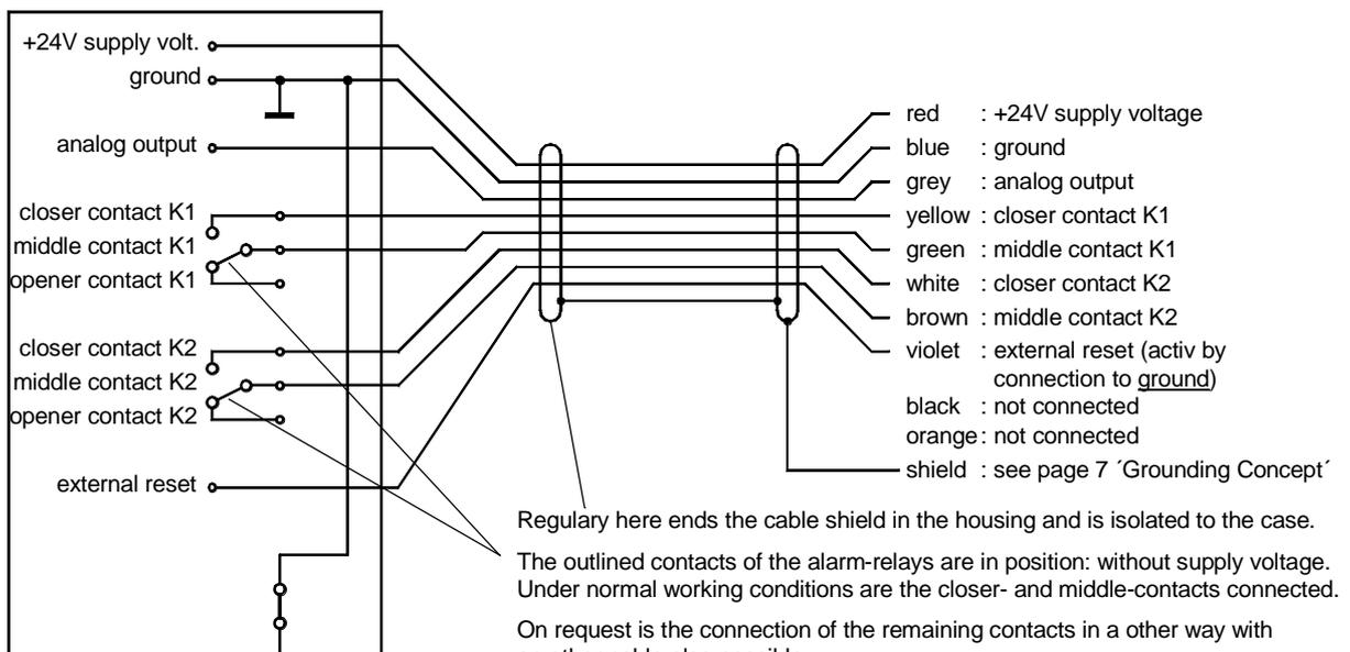
Regularly here ends the cable shield in the housing and is isolated to the case.
