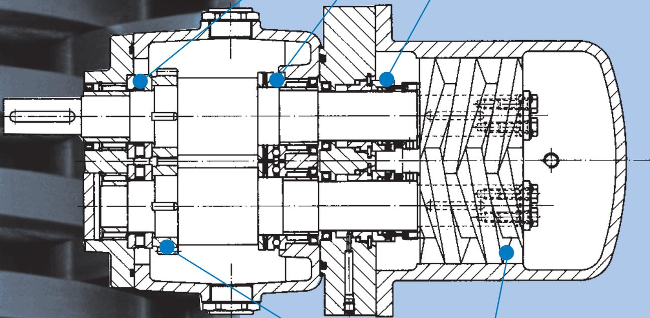
The special profile of the spindle flanks results in **continuously and nearly pulsation-free pumping, high efficiency, good NPSH-values and constant pressure course.**
