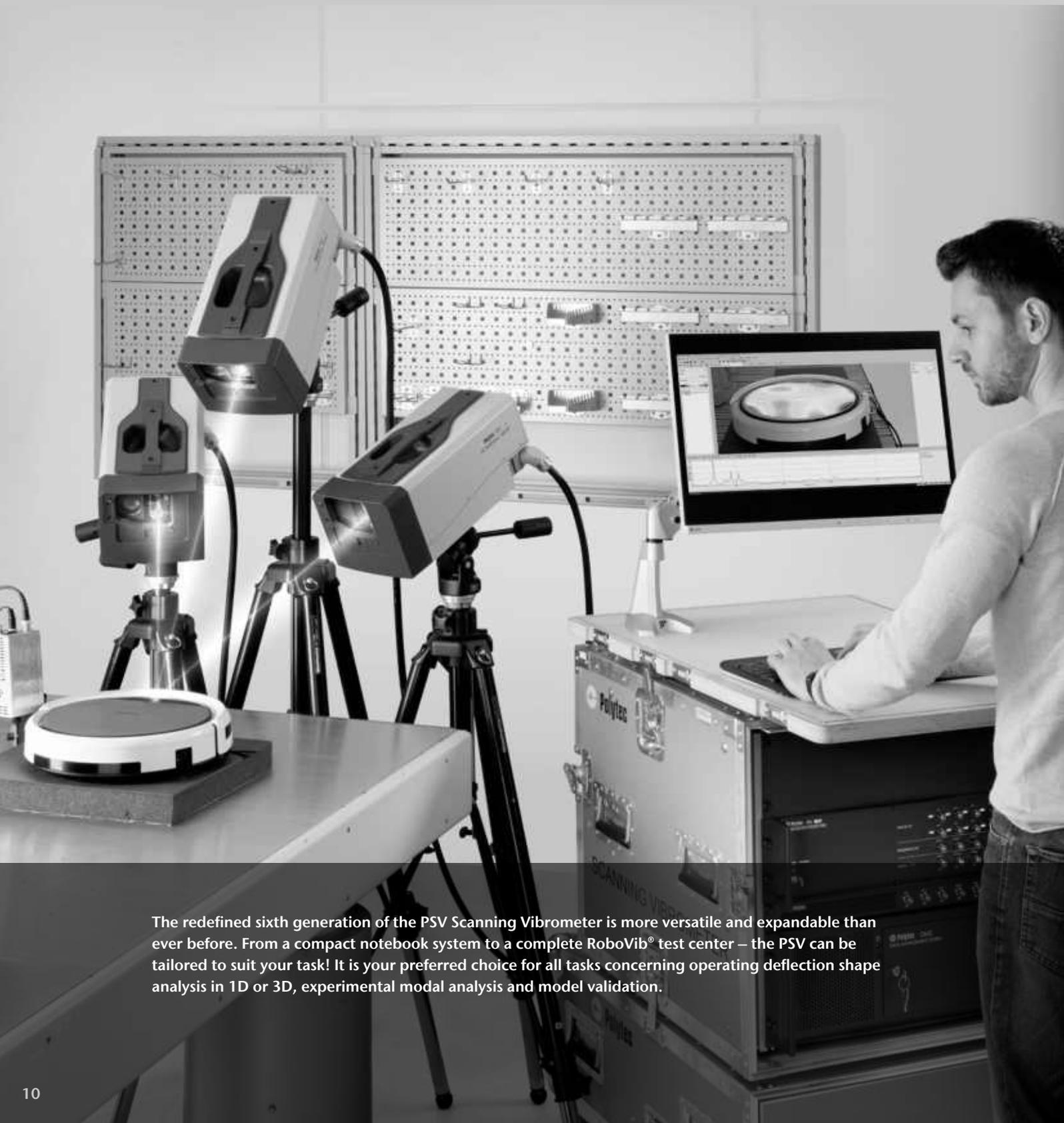
The redefined sixth generation of the PSV Scanning Vibrometer is more versatile and expandable than ever before. From a compact notebook system to a complete RoboVib® test center – the PSV can be tailored to suit your task! It is your preferred choice for all tasks concerning operating deflection shape analysis in 1D or 3D, experimental modal analysis and model validation.
