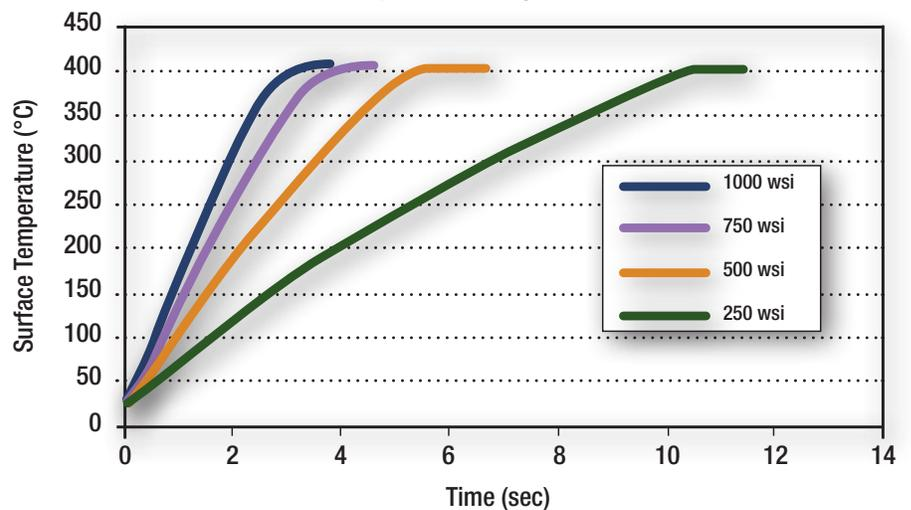
*ULTRAMIC temperature ramp rate as a function of watt density. Test completed using Watlow's SERIES F4 temperature controller.*
