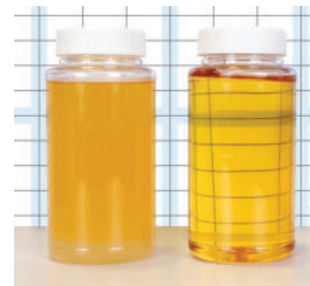
Contaminated Fuel - emulsified water with free water at bottom
