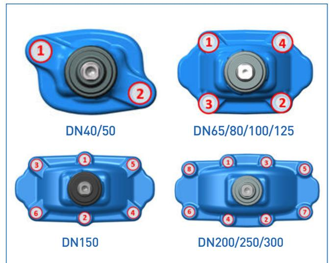
Figure 3: Assembly order for body/bonnet bolts
