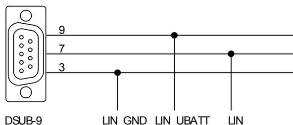
**Fig. 4-2** Power Supply at the LIN Bus
