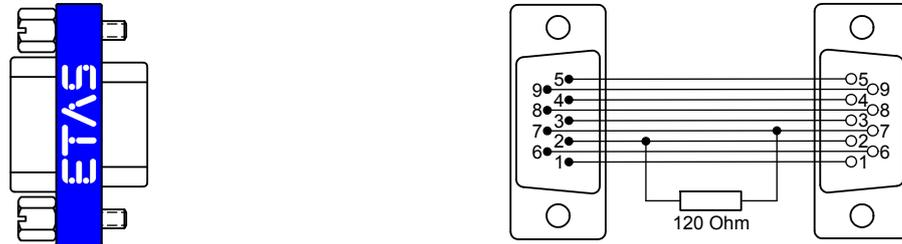
**Fig. 8-18** CBCX131-0 Termination Resistor
