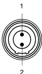
Fig. 7-2 Power Supply Interface (7-29V)
