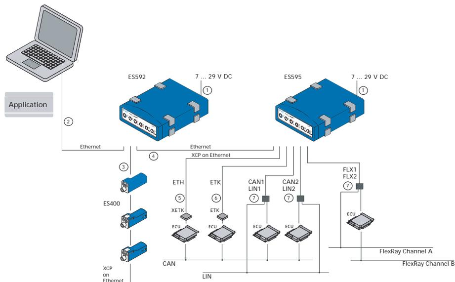
**Fig. 5-4** ES592.1 and ES595.1 with ES400 modules, XETK, ETK and vehicle buses
