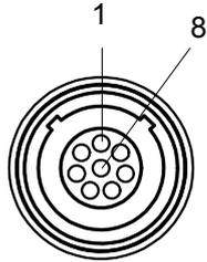
**Fig. 7-6** CAN/LIN Interface (CAN1/LIN1 and CAN2/LIN2)
