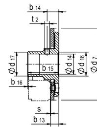
Connecting part out of non-magnetizable material
