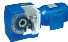
The helical gears of helical worm gear units are made of highly alloyed steel with case-hardened teeth. Optimised geometries and precise shaft alignment due to the UNICASE principle provide excellent load-bearing capacity, long operating life and low noise.
