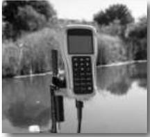
The new FlowTracker2 (FT2) handheld Acoustic Doppler Velocimeter (ADV®) has all the technology you have grown to know and trust with the original FlowTracker, but now comes with functional, modernized features (Bluetooth, GPS and large color screen, to name only a few) based on the evaluation and feedback from hydrologists, researchers and scientists who have made the FlowTracker their instrument of choice.
