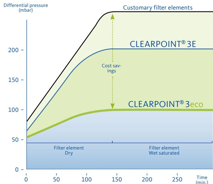
The operating costs for the CLEARPOINT® 3eco filter can be considerably lowered. The graphic illustrates them on an example of the S040 filter with filter rating S with energy-optimised volume flow.
