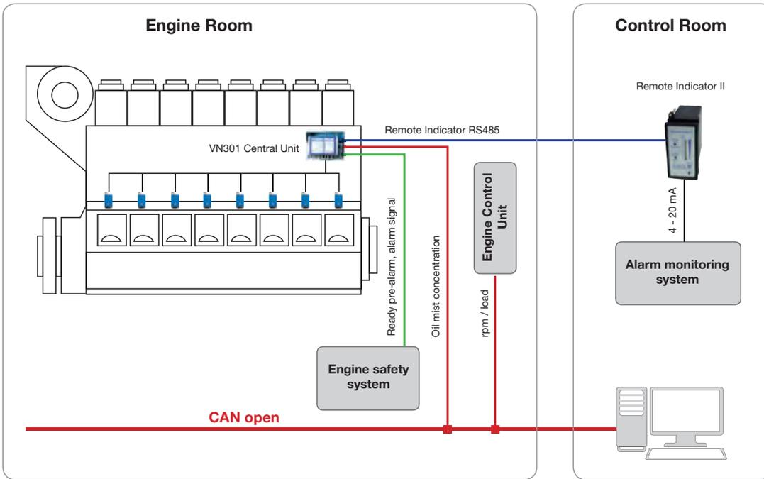
sensors ensure that the crankcase is monitored.
